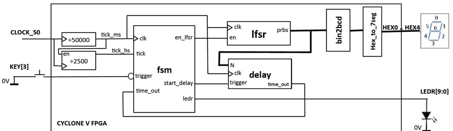
In the above diagram, all signals on the left of the block are inputs and the signals on the right are outputs.
