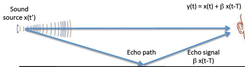
Such simple echo can be implemented as signal flow graph as shown below. This involves three components: a delay block that delays  $x(t)$  by  $K$  sample periods; a gain block which multiplies the delayed signal by the factor  $\beta$ ; and the adder.
